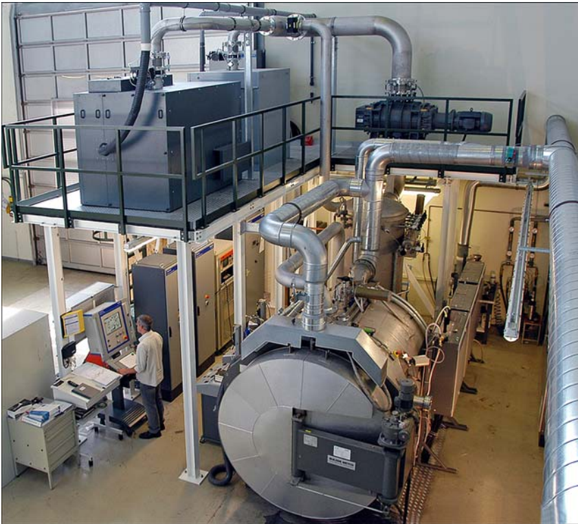
Fig. 1 Vacuum plasma spray unit at Forschungszentrum Jülich GmbH that recently has been upgraded for low-pressure plasma spraying (LPPS) with working pressure range down to 1 mbar
